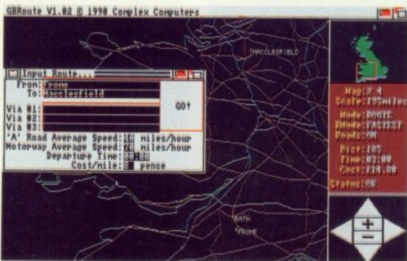
Click on the New button and this requester appears. Now enter your start position and required destination, click on the GO gadget and et voila - the fastest route between Frome and Macclesfield
